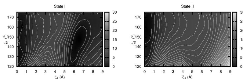
**Fig. 3.** Free energy profiles of molecular shuttle (in kcal/mol) for state I and II in NaCl solution (contour spacing is 1 kcal/mol)
