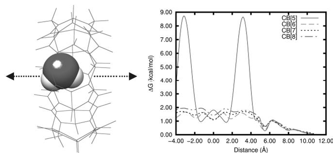
**Fig. 4.** (left) scheme of water transit through the CB[x] cavity; (right) corresponding free energy profiles
